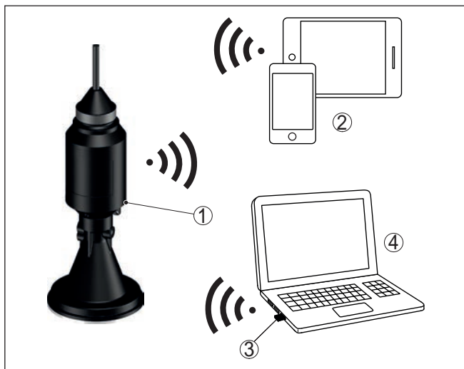
Fig. 5: Wireless connection to standard operating devices
