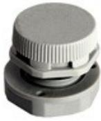
A semi-permeable filter located next to the cable glands on the underside of the H520's level box ensures air pressure equalization between the outside environment and the H520's internal sealed compartment, which is important not only for correct level measurement, but also for preventing condensation inside the unit during temperature changes common to day and night time.
