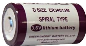
If the level gauge includes a built-in GSM communication module, which requires higher current consumption for data transmission, then the level gauge must be powered by a spiral type lithium battery 3.6 V / 13 Ah, which provides a short-term peak current of up to 1.8 A (battery type ER34615M).
