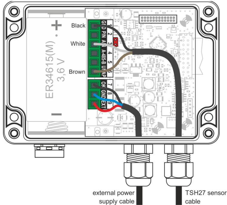
**Remark:** *The TSH27 and TSH35 or LMK809 sensors have interchanged power and signal wire colours. Therefore, pay due attention to the sensor connection!*
