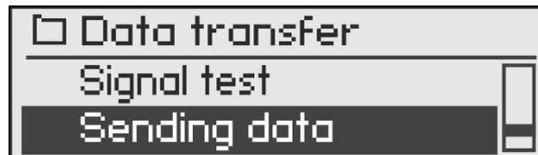
After the "Send data" procedure is started, the device is first logged into the GSM network.
