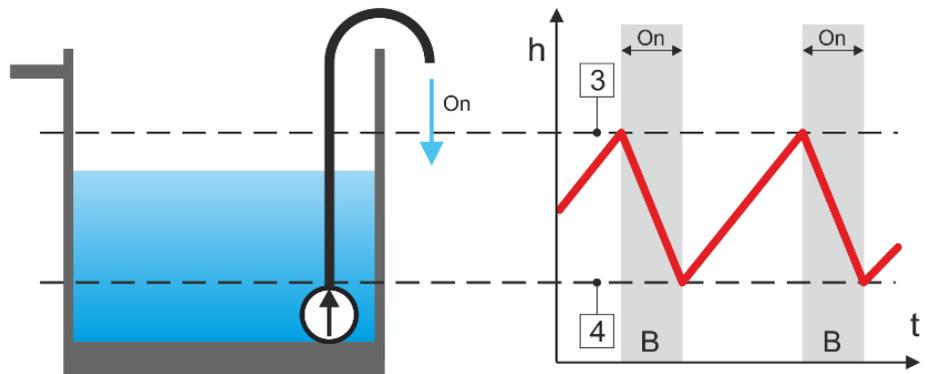
**Example 7.** Setting the switch-on [3] and switch-off [4] levels for controlled pumping of water from the sump by the submersible pump.
