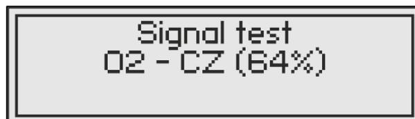
The level gauge automatically switches to the basic display mode after about 10 seconds of displaying the GSM field strength.
