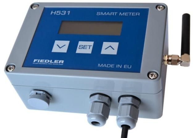
For the actual mounting of the H531 unit, there are 4 mounting holes in the bottom of the level gauge box that are accessible by removing the top of the display box. When installing the level gauge, the flat cable connecting the bottom and top of the H531 display unit can be disconnected for ease of installation.
