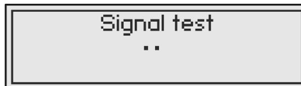
After the device is logged into the GSM network, the name of the GSM operator and the GSM field strength are displayed on the device display.
