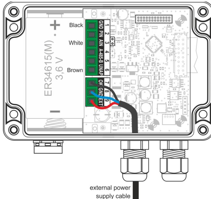
**Setting jumpers** The two previous sensors also have different type of analog output signal (0..5 V for TSH27, 4-20 mA for LMK809 and TSH35) and therefore it is necessary to set the correct position of jumpers 6 and 7 from the picture on page 6. 14.
