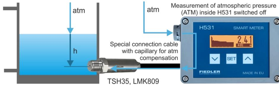
*The principle of level measurement using a pressure compensated level sensor*
