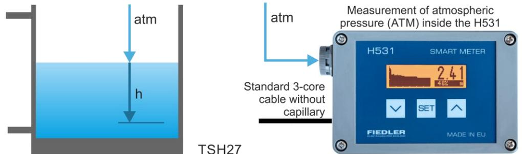
*The principle of level measurement with an absolute level sensor*
