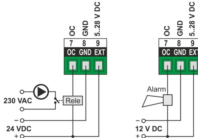
*Example of connecting an external relay or audible siren to the terminals of a level gauge.*
