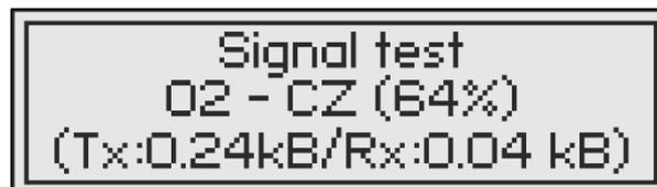
During the data transfer to the server, the continuous volume of sent (Tx) and received (Rx) data in kB is displayed on the bottom line.
