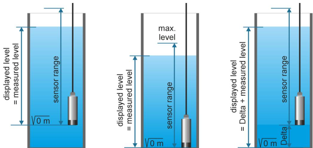
Measurement by immersion depth Level measurement from the bottom
