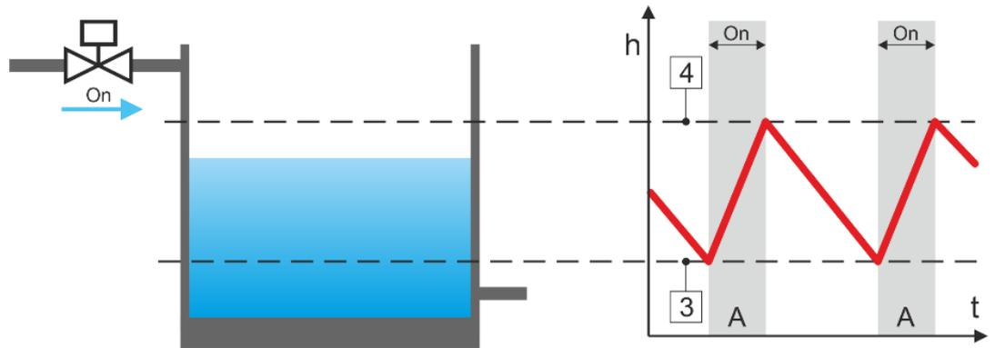
**Example 6.** Setting of the switch-on [3] and switch-off [4] levels for controlled water supply to the sump by means of a solenoid valve.
