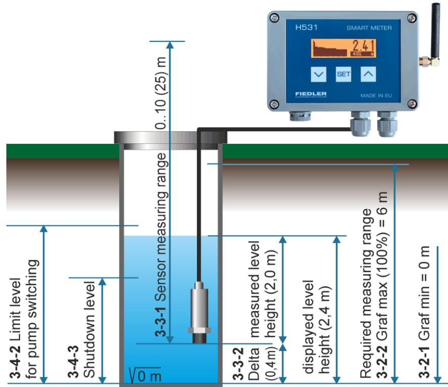
Graphical representation and meaning of H531 parameters for display and control.
