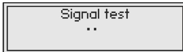
After the device is logged into the GSM network, instead of flashing dots, the name of the GSM operator is displayed in the middle of the display frame and the currently measured GSM field strength in brackets.
