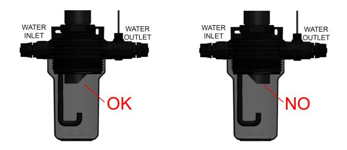
Install the probe in the pss8 respecting the position shown in the figure above.
