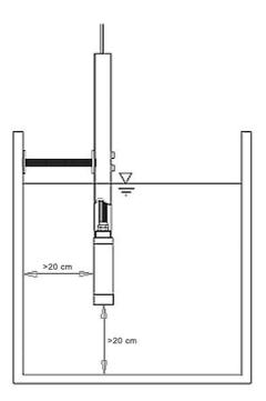
Install the probe in the tank so that it is immersed for at least 20 cm and the distance from the walls and the bottom of the tank is not less than 20 cm.
