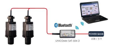
The instruments with HART® output can be connected to a PC via Bluetooth® wireless connection using a UNICOMM HART®-USB-Bluetooth® modem (SAT-504). We can provide power supply for the system with a USB power bank connected to the UNICOMM modem.
